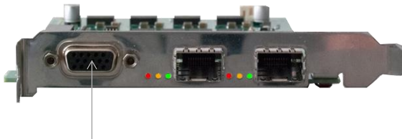
15-pin D-Sub 15 socket (Front GPIO) for triggering and synchronizing peripheral devices, including two TTL GPOs
