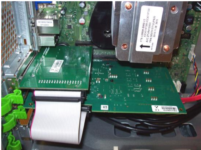
marathon frame grabber and trigger board being connected via 34-pin flat cable
