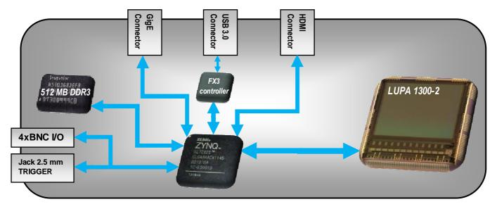
These abilities are used to perform automatic image triggering, lossless compression or sub-sampled images and for instance images binarization, on the fly data generation like blobs edge or barycenter coordinates.
